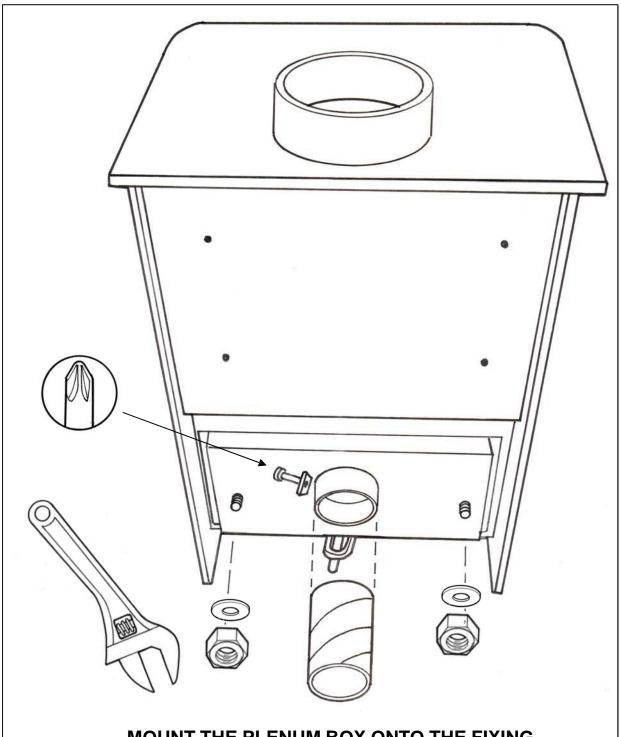
MOUNT THE PLENUM BOX ONTO THE FIXING STUDS AND SECURE WITH THE 2 X M8 NUTS AND WASHERS.
