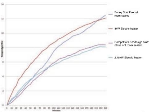
The graph shows a real life comparison between a Burley 5kW room sealed stove and another leading 5kw stove which cannot be room sealed. Before the room even reached 21 degrees the non-room sealed stove was sucking heat from the room faster than it could put it in. Burley's stove however warmed the room up to a toasty 28 degrees and showed no sign of slowing down, 50% extra warmth for the same amount of fuel.
