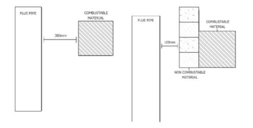
If a wooden beam is to be fitted, the distance from the rear of the beam to the flue MUST BE 3 times the diameter of the flue e.g. 380mm if using a 125mm flue pipe. If non-combustible material is placed between the flue and the rear of the beam this should be at least 100mm thick.
