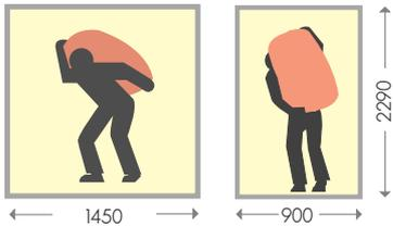
Any access way or passage between lorry and storage should have a minimum clear height of 2290mm (unobstructed by light fittings) and a minimum width of 900mm.
