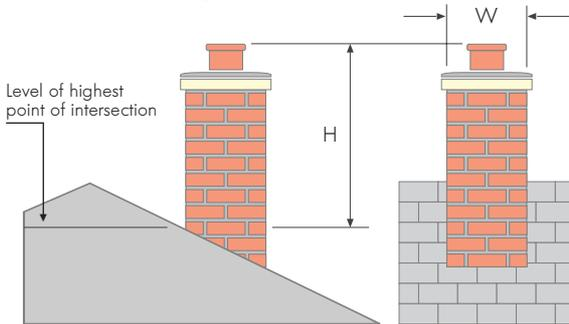
H should not exceed 4.5xW Note: W is the least horizontal dimension of the highest point of intersection with roof surface, gutter etc, and H is measured to top of any chimney pot or terminal
