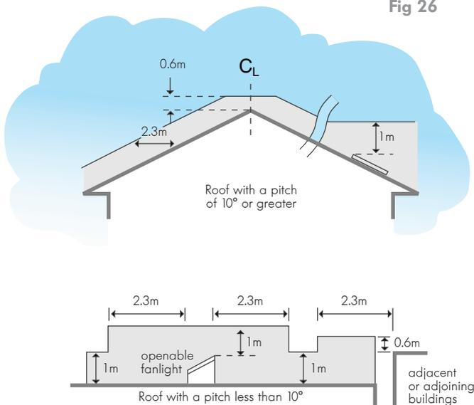
Flue outlet should terminate outside the shaded area
