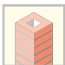
FLUE - provides ventilation and reduces risk of condensation. The chimney acts as a thermal store which helps to even out air temperature variations.
