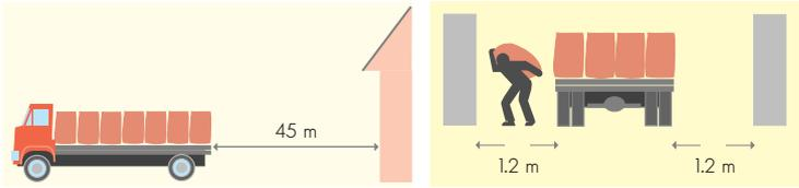
At the unloading point a clearance of 1.2m on each side of the lorry is desirable
