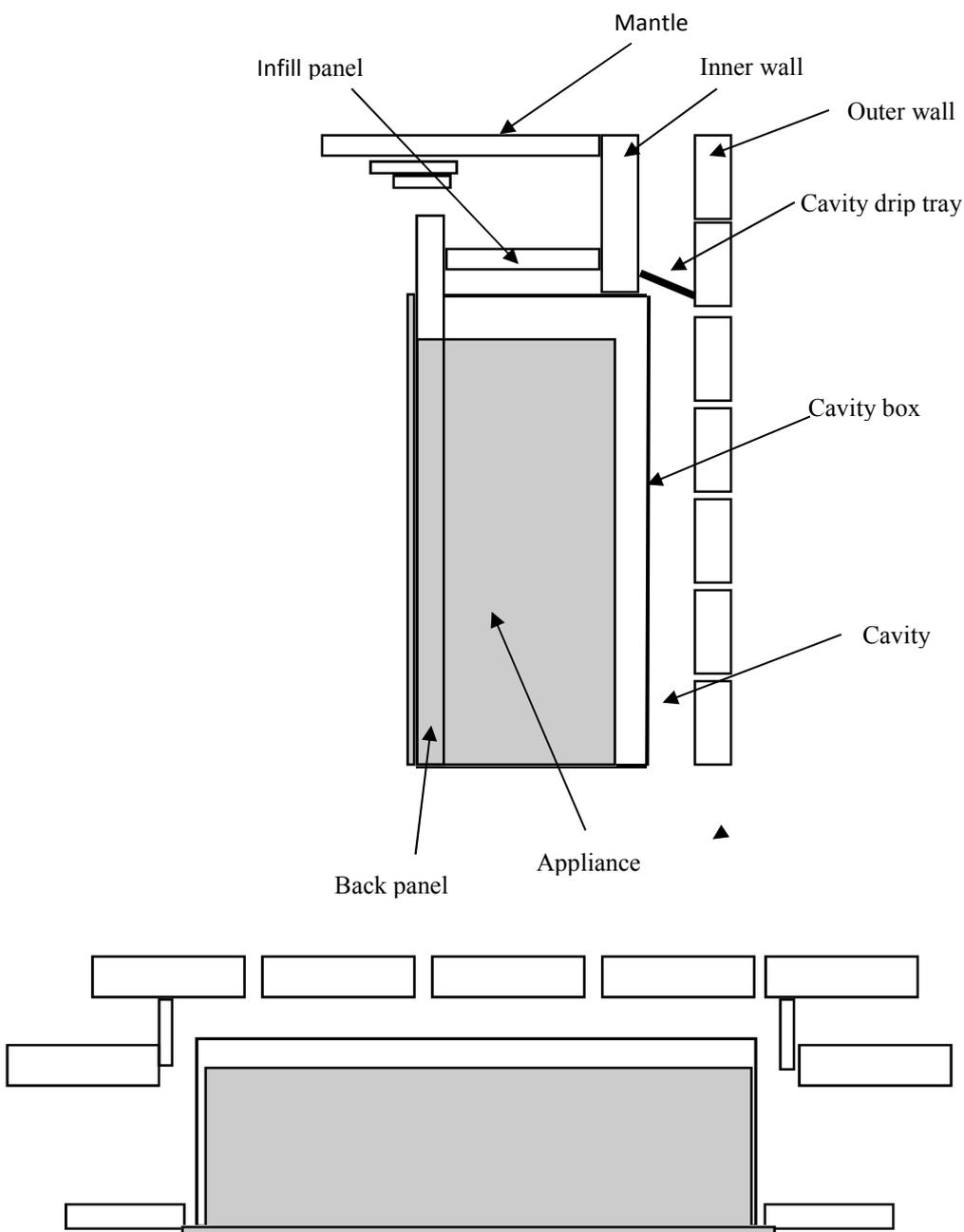
7.2.1 Decide on the location of the appliance taking account of any wiring or pipe work that may be running within the wall, and mark the wall for the fire place opening to the dimensions specified in section 5b.
