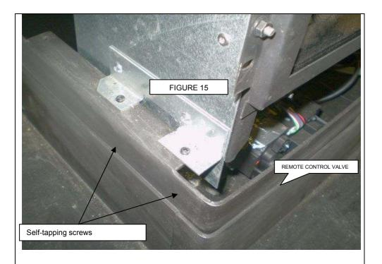
Once the balanced flue gas fire assembly is screwed to the base casing (as shown above), the next stage is to prepare the fireplace for the installation of this 'sub assembly'.
