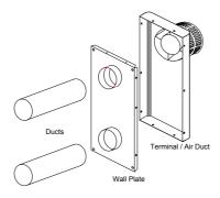
FIGURE 13 PARTS OF THE FLUE KIT
