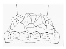
Top ceramic fitted on top of front
