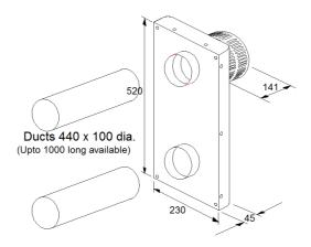
FIGURE 11 Flue Pipe and Air Box with terminal (all dimensions in mm)
