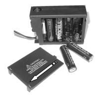
FIGURE 9 RECEIVER BATTERY REPLACEMENT
