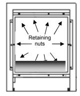
FIGURE, 23 GLASS FRAME RETAINING NUTS
