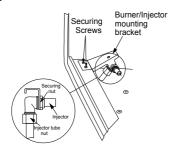
Figure 25 INJECTOR DETAILS
