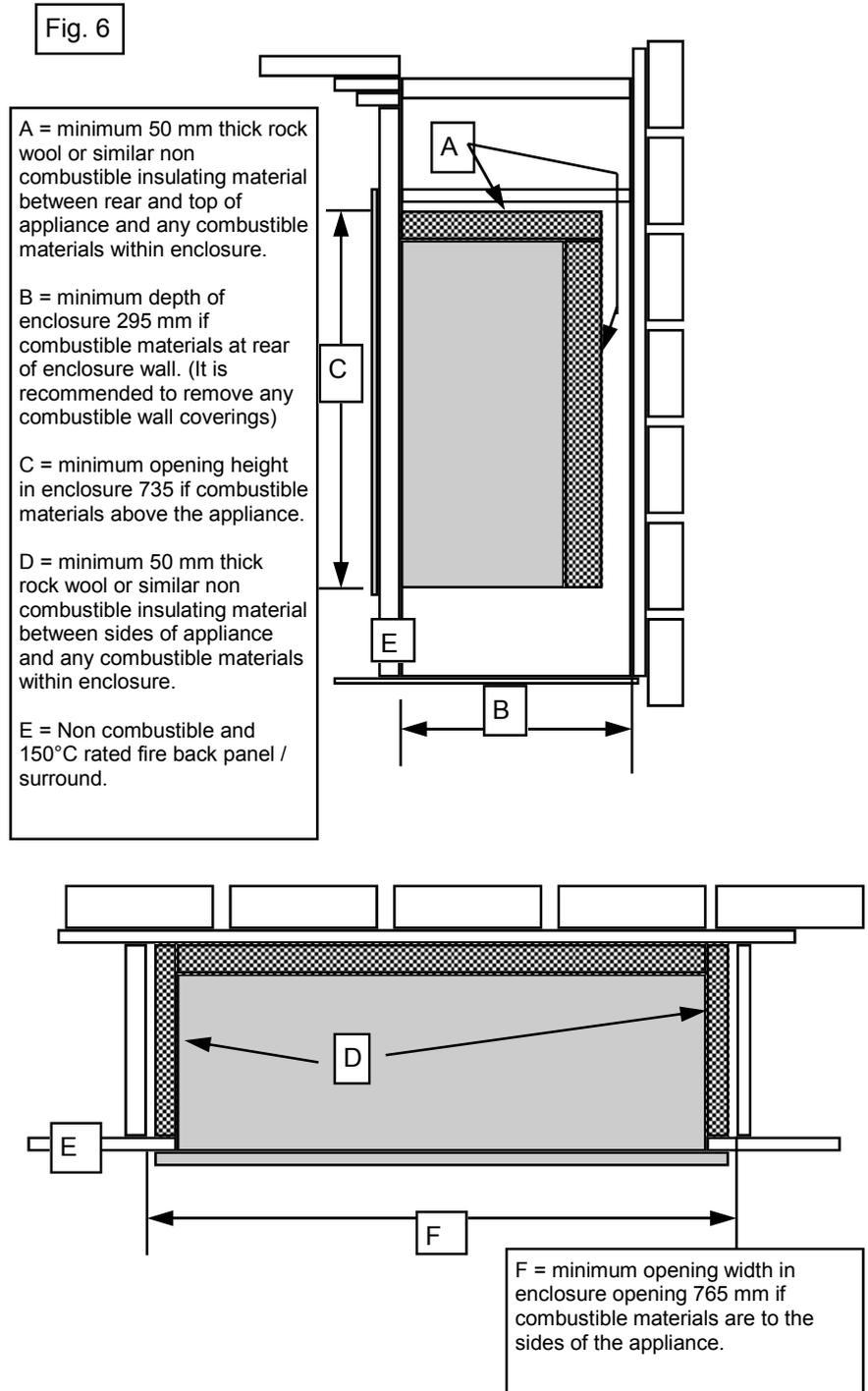
7.1.4 A suitable non combustible support platform shall be constructed within the enclosure for the appliance to sit upon.
