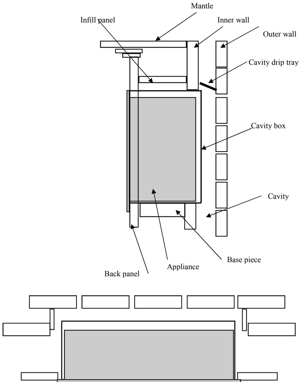
7.2.1 Decide on the location of the appliance taking account of any wiring or pipe work that may be running within the wall, and mark the wall for the fire place opening to the dimensions specified in section 4.2.
