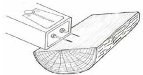
Simply putting the contact pins onto the surface will not give an accurate reading, as it may tell you that the surface is dry whilst the interior of the log may well be damp.
