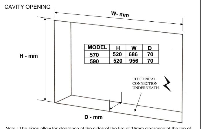
Note : The sizes allow for clearance at the sides of the fire of 15mm, clearance at the top of 20mm and 5mm at the back.
